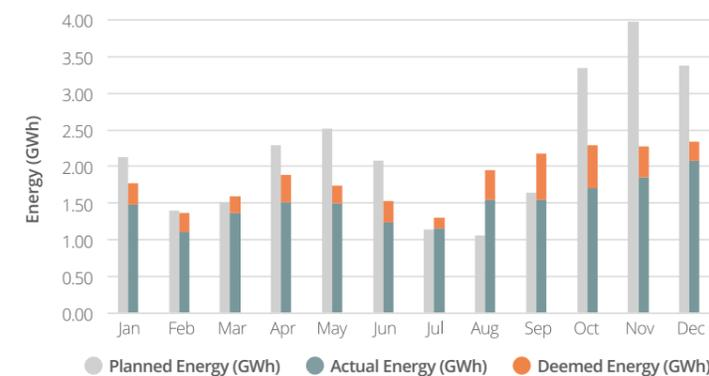
Figure 20 | Ndugutu SHP – Planned versus Actual Energy Output (2022)
